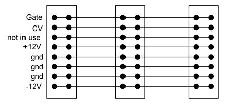
Pin connectors, power supply board
