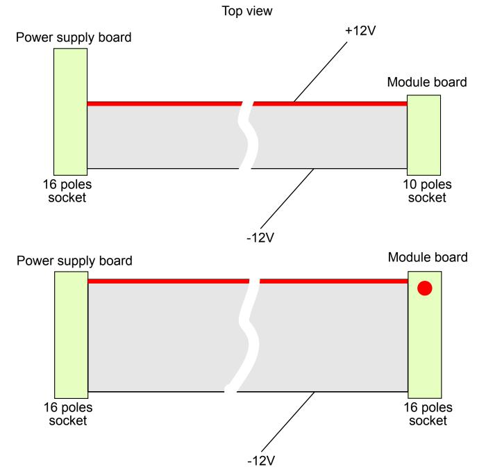
ATTENTION! Be careful with connecting the ribbon cable to the power supply board. Reversing of the ribbon cable connector can cause the destruction of the wrong connected module(s).
